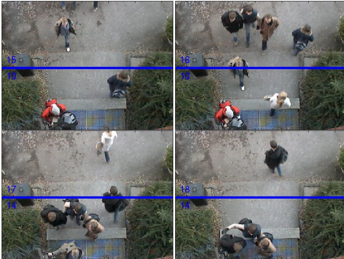
People entering and exiting entrance. Number above line gives number of people crossing the line going out. Number below line gives number of people crossing the line going in.
