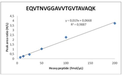
Figure 2. Linearity of the alpha-synuclein SRM assay determined by using heavy labeled peptides spiked into a pooled tissue sample at various estimated concentrations (6.25–200 fmol/ $\mu$ L). doi:10.1371/journal.pone.0110804.g002
