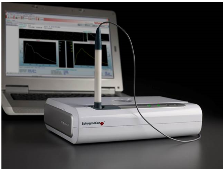
Figure 2. This device (SphygmoCor ® ) was used for the assessment of c-f PWV and central BP in the MDC-CV reexamination.
