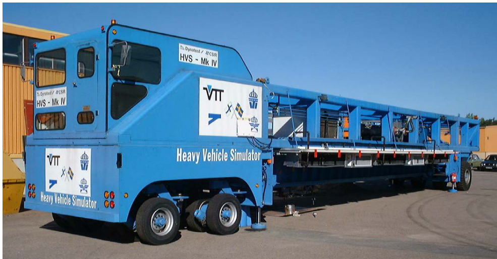
Figure 2-2. The accelerated pavement testing facility called heavy vehicle simulator (Wiman, 2005).
