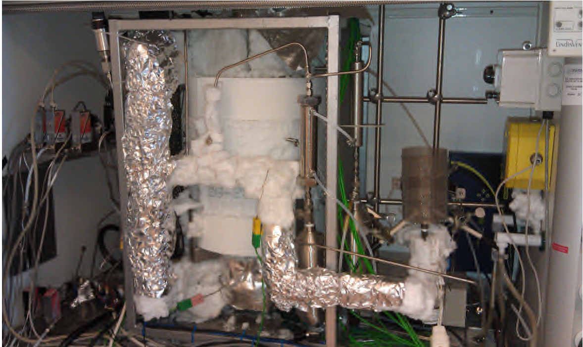
Figure 8: Laboratory reactor with mass flow controllers, flame cage and analysers.
