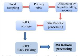
**Fig 4** Schematic illustration of our work flow with electronic surveillance and LIMS integrated system.
