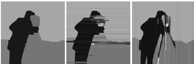
Figure 8.4: Result using the Potts model with 64 labels. To the left the solution obtained by \alpha -expansion is shown, followed by the row and column solutions of Fig. 8.1 after 500 iterations. Running 10000 iterations did not improve the solutions significantly.
