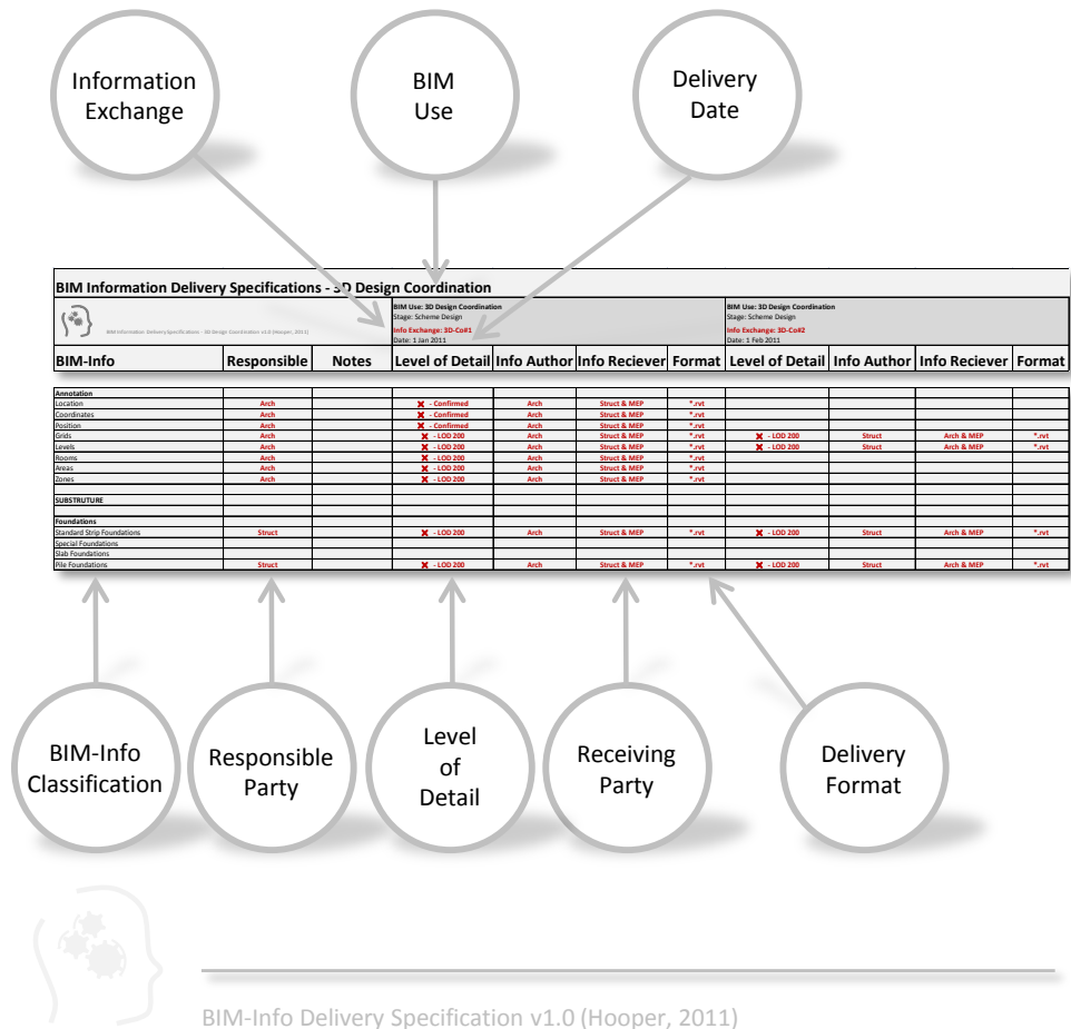
Figure 11: BIM-Info Delivery Specification – Constituent Parts
