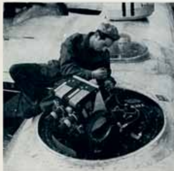
PREFACE TO PRECISION. On a Boeing F-13 plane altered for use as a photographic ship two movie picture cameras are installed in one of the plane's gun turrets. These cameras were controlled from the top fire control blower shown in the background by the same sighting and firing mechanism normally used with the plane's machine guns. Shows here at Roswell Field, New Mexico, are Corporal Harold Johnson, outside the plane, making adjustments on the camera, while Sergeant Henry R. Zarnoff, near the controls in the top fire control blower. In the background can be seen another turret, started cover in place, housing a similar movie picture camera installation.
