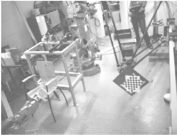
Figure 5.25 View out of the camera: The robot with the calibration pattern (to the right in the picture). To the left in the picture, obstacles, e.g., experiment equipment and and ABB IRB 2400 robot can be seen.
