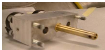
Figure 7 Designed injector mouthpiece
