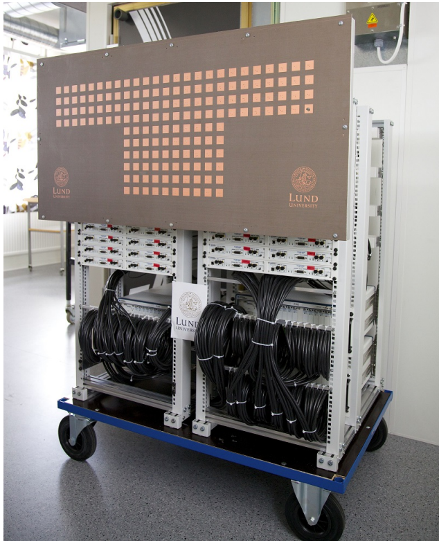
Figure 3.1: The BS of the LuMaMi testbed. In the front sits an antenna array made out of 160 patch antennas.
