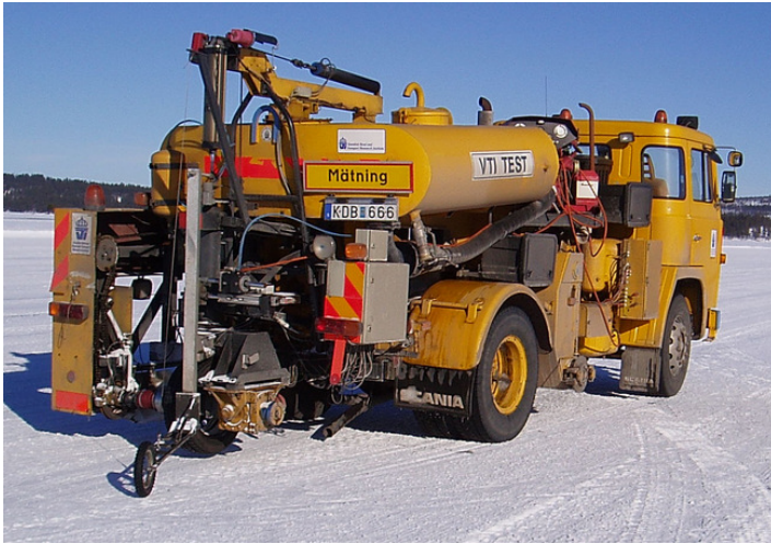
Figure 10.1 VTI's BV12 measurement vehicle at Colmis proving ground, Arjeplog, Sweden. This vehicle has an additional wheel for which the normal force can be set, and sensors to determine the resulting tire forces, allowing the friction between the tire and the road surface to be measured. Such measurements were used to validate the brush model.
