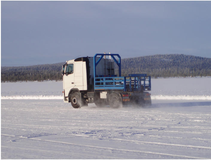
Figure 10.12 The FH12 test vehicle performing a maneuver on a frozen lake at Colmis proving ground. Note that the surface consists of a thin layer of snow on top of uneven ice. The wide variety of possible driving surfaces highlights the problems of classification-based estimation techniques.
