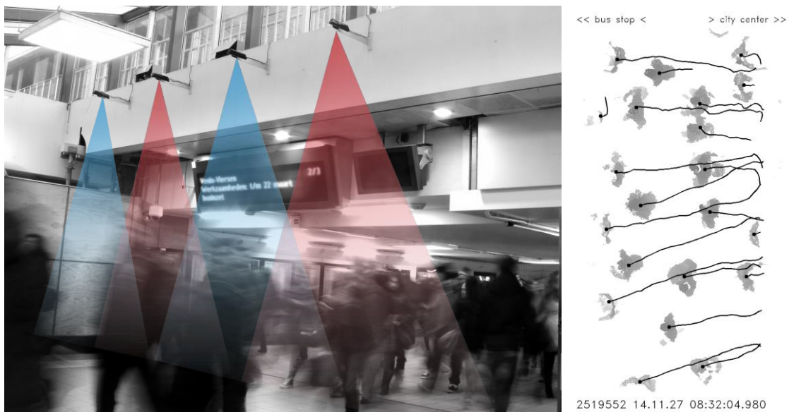
Figure 2. (top) Crowd tracking experiment at the Metaforum Building, Eindhoven University of Technology; setup sketch, example of collected trajectories and related depth maps (figure from (Corbetta et al., 2017b)). (bottom) Crowd tracking experiment at Eindhoven train station with four Kinect sensors: snapshot and sample depth map with trajectories. In both cases depth maps have grayscale colorization (figure from (Corbetta et al., 2016b)).
