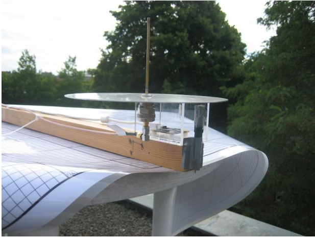
Figure 7.6 IMU and dipole antenna with ground plane mounted on the wooden stick.
