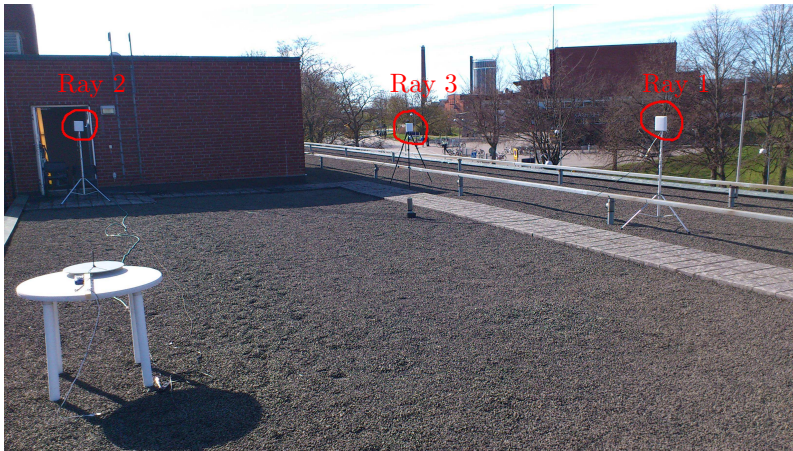
Figure 7.7 The test area with the table holding the IMU and receiver antenna closest to the viewer. The three transmitter antennas acting as scattering objects are marked in red.
