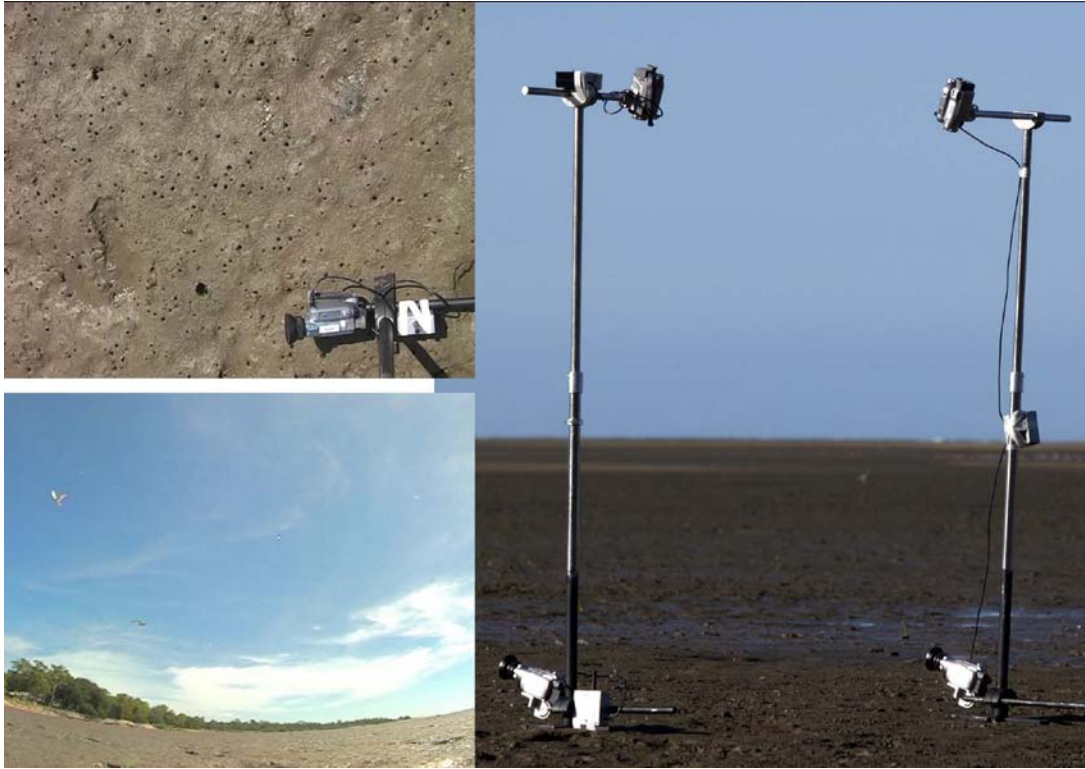
Fig. 1: The synchronised four-camera setup. The two lower cameras were fitted with fish-eye lenses to observe a field of view of approximately 50° by 80° each. The top cameras pointed down to observe crab behaviour on the mudflat. Sample images are shown next to each camera.
