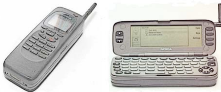
Figure 6. The Nokia 9000 Communicator, launched in 1996. Being a merger of a mobile phone and a PDA, it is an example of an early smartphone. To the right, the phone is up folded and the extended screen and keyboard is visible (picture Pdadb (2011b)).
