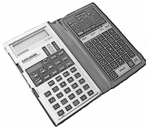
Figure 3. The Casio PF-3000 Digital Diary launched in 1983 and considered one of the first PDA's (picture Pdadb (2011b)). In this picture with its foldable plastic cover.
