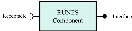
Figure 2. Graphical representation of a RUNES component. Interfaces are sets of functions, variables and associated data types that are accessible by other components. Receptacles are required interfaces by a component.
