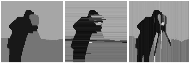
Figure 8.4: Result using the Potts model with 64 labels. To the left the solution obtained by \alpha -expansion is shown, followed by the row and column solutions of figure 8.1 after 500 iterations. Running 10000 iterations did not improve the solutions significantly.
