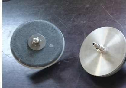
Figure 12 Typical ceramic diffusers for ozone. The darker part of the left diffuser is the porous ceramic material dispersing the gas, and the diffuser on the right is overturned to show the connection point of ozone (middle threaded connection).
