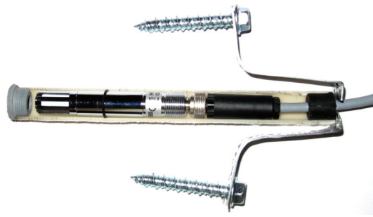
Figure 26. Photograph of the measurement setup with the casing pipe split in half.
