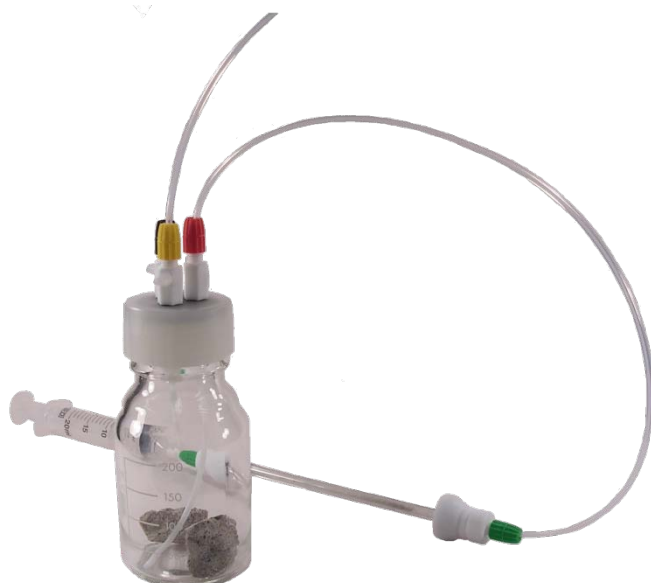
Figure 1. Flask with two concrete pieces during sampling. Connected via Teflon tube to a TENAX tube and a plastic syringe.
