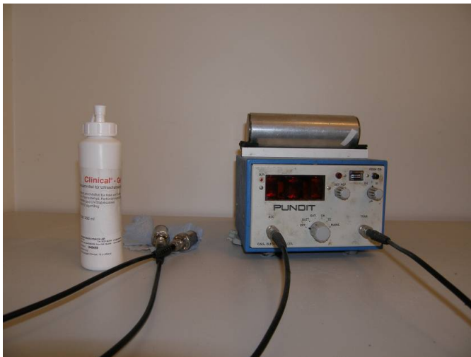
Figure 31 The contact gel, reference material and speed of sound apparatus.
