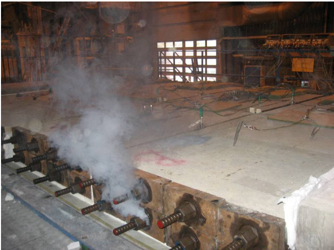
Figure 22: The loading system on the side without load cells during fire test.
