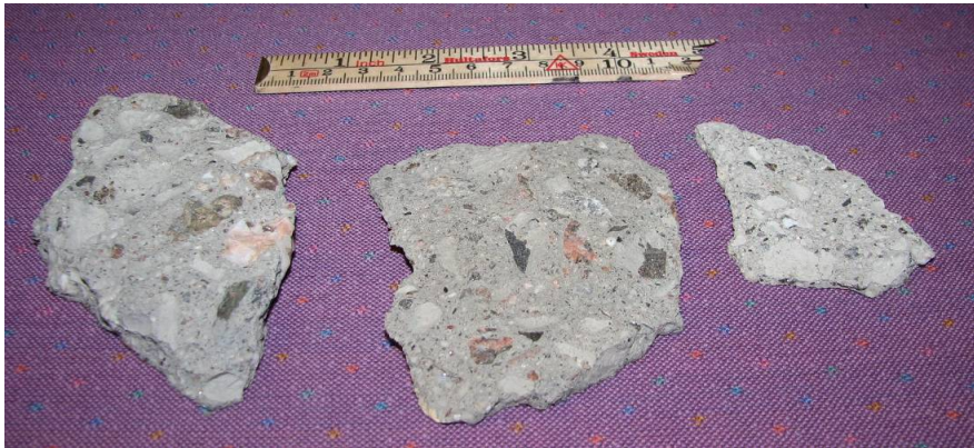
Figure 39 Spalled material from the surfaces of three different concretes.
