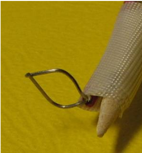
Figure 6 Welded thermocouple wire, diameter 0.5 mm.
