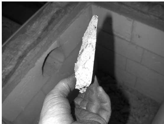
Fig. 5 This is some of the material spalled of form specimen “A, 3 month, 5%”.
