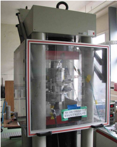
Figure 34 The equipment for measurements of mechanical properties at high temperature at CSTB in France.
