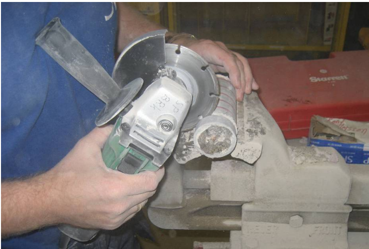
Figure 12 The author is notching of the specimens.
