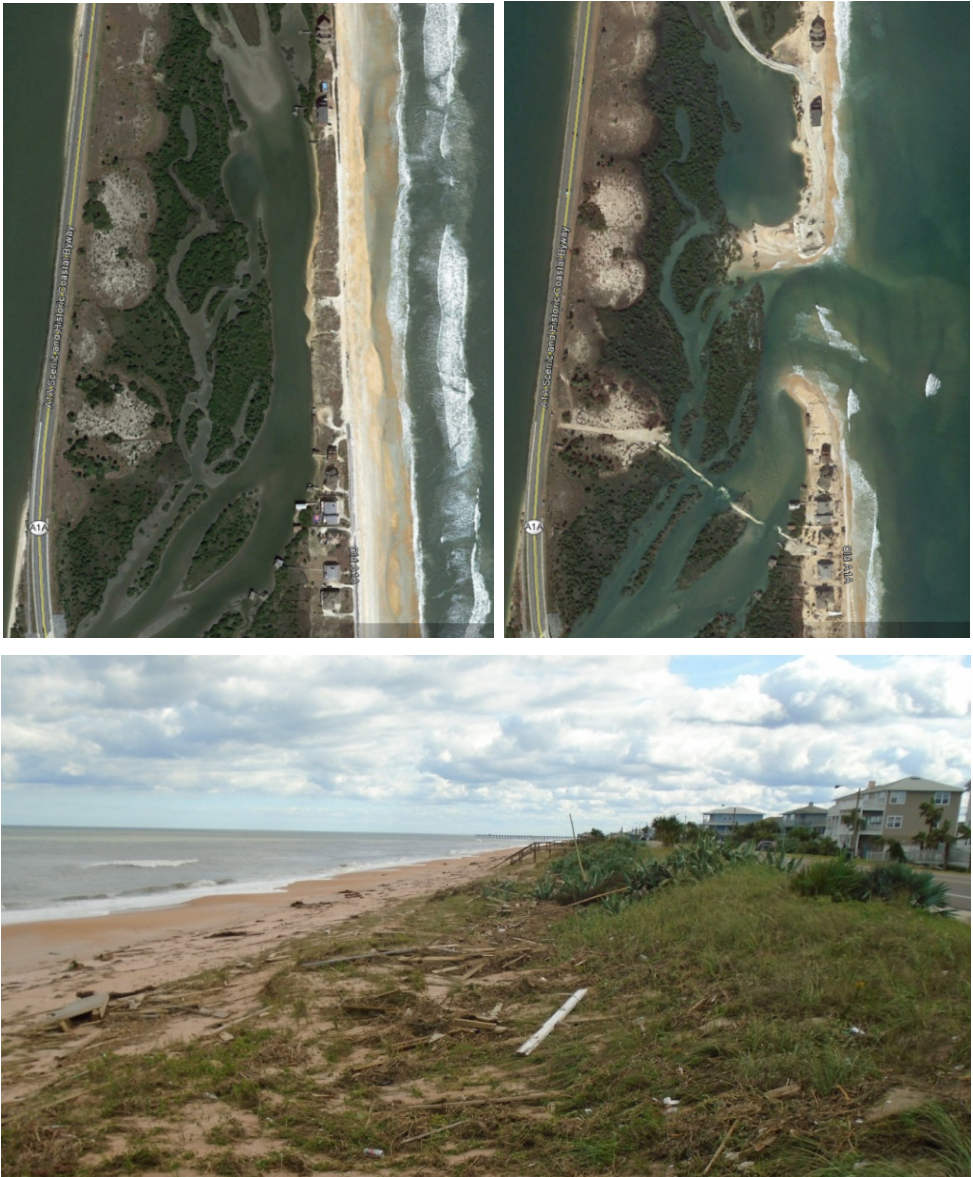
Figure 32: Top left and right: Repeat GoogleEarth images showing the creation of a new inlet. Top Left: February 2016, pre-Hurricane Matthew; Top Right: Nov, 2016, post-Hurricane Matthew. Source: Google, 2017. Bottom: a well vegetated fore-dune in northern Flagler Beach helped mitigate erosion during the storm, while leaving exposed roots and stems which, as they grow, will help initiate the dune recovery process. Source: Author's photo: 2016.
