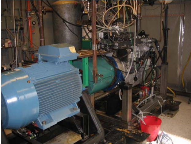
Figure 5 The Scania D12 single-cylinder test engine used in the study.
