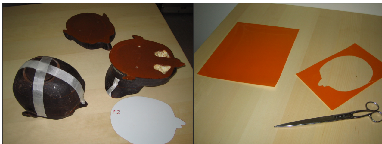
Figure 1. The anatomical head phantom and the Gafchromic® film cut to fit between the different layers of the phantom.
