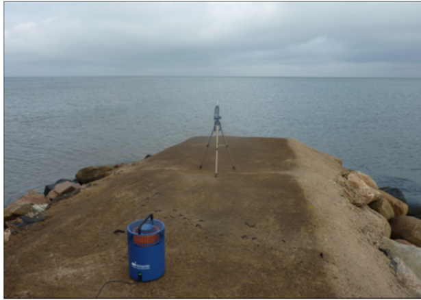
Picture 6. Measuring the sound level on a pier.
