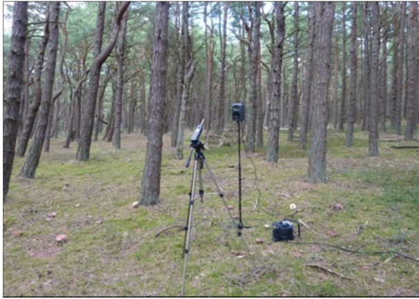
Picture 1. Measuring sound level at 1 meter.
