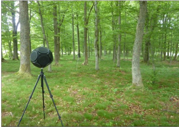
Picture 5. Measuring impulse response in beech forest.
