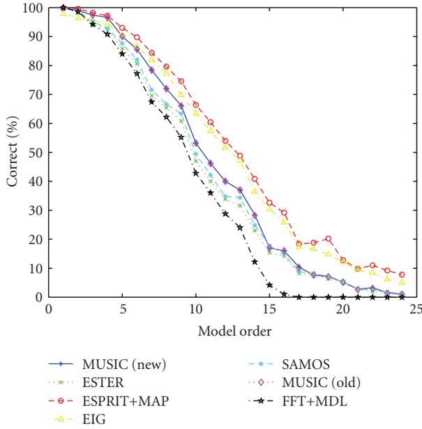
FIGURE 4: Percentage of correctly estimated model orders as a function of the true order with SNR = 20 dB and  $N = 100$ .
