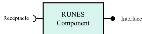
Figure 2 Graphical representation of a RUNES component. Interfaces are sets of functions, variables and associated data types that are accessible by other components. Receptacles are required interfaces by a component.
