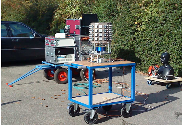
Figure 3.5: RUSK Lund MIMO channel sounder RX unit with cylindrical probe array antenna.
