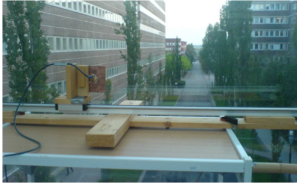
Figure 3.3: Linear positioning robot with TX probe antenna.
