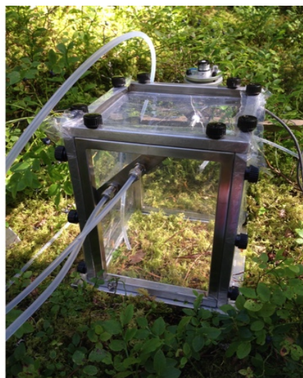
Figure 4. A soil chamber was placed on the frame with tap water filled in the channel to make the frame airtight.
