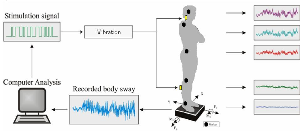
Figure 3: Illustration of the posturographic measurement system. The illustration shows the position of the movement markers in black and examples of the data captured simultaneously by both Zebris and the force platform.
