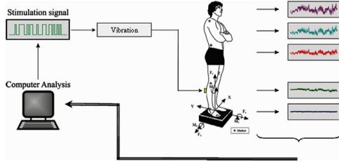
Fig. 1. Schematic picture of the measurement setup and placement of the five Zebra markers attached on a subject. The marker locations are shown by small circles.
