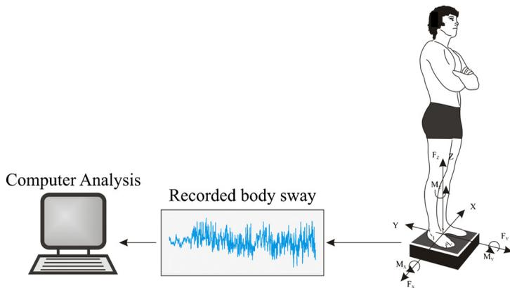
Fig. 1. Schematic of the measurement system and force platform, with recorded forces and torques marked.
