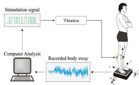
**Fig. 1** Schematic illustration of the test setup
