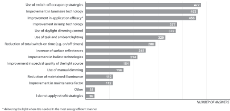
Figure 5.2 Main retrofit strategies used by lighting practitioners (source: IEA-SHC Task 50 Subtask C)
