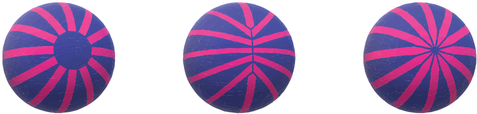
Figure 5 The problem of covering a sphere with fibers. Left: Equally wide straight fibers (stripes), laid from one pole to the other, cannot cover the poles without overlapping. They would leave gaps. Center: Example of organizing the fiber ends in a ‘line’ suture. Left: Umbilical sutures require fibers to reduce their widths before reaching the pole.
