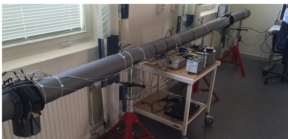
Fig. 4: A 4.5 [m] prototype with two directional couplers was setup and used for controller development and experimental evaluation.
