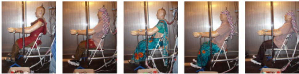
Figure 4: The thermal manikin Tore in the tested work clothing ensembles at the Thermal Environment Laboratory, Lund University (Photos by Kalev Kuklane).
