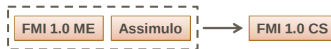
Figure 4.6: By bundling ASSIMULO together with an FMU for model exchange an co-simulation FMU is created.
