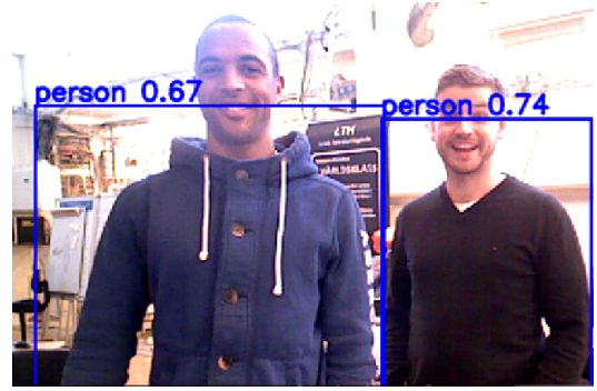
Fig. 11. The figure shows the classification done by the YOLO9000 network using an ASUS Xtion camera. The bounding boxes show where the persons are and the text above them shows what type of object they are and the corresponding certainty.
