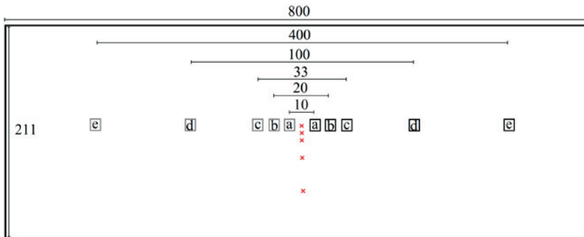
Figure 12. Layout of the concrete floor slab, transducers, and boreholes. Dimensions are given in cm. The transducer pairs denoted by a-e in the figure were used for signals with frequencies 500, 250, 150, 50, and 3.1 kHz, respectively. The transducers to the right of the center were used as transmitters and those to the left as receivers. The red crosses indicate the location of the boreholes. The boreholes are located 0, 5, 10, 20 and 40 cm from the centerline, between the transducers. The sketch is not to scale and the transducers were placed slightly off-center on the slab due to other instrumentation on the concrete. Image from Fröjd and Ulriksen (2017).
