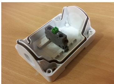
Figure 2.18 Snap-fit experiment: a part of an emergency switch is to be assembled; the dark-gray electric switch is to be fastened by snapping it to the rail of the light-gray box.
