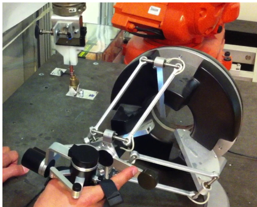
Figure 2.11 Peg-in-hole setup: (Front) Master side with Omega-7 haptic interface. (Back) IRB140 robot with metal pipe held in the gripper.
