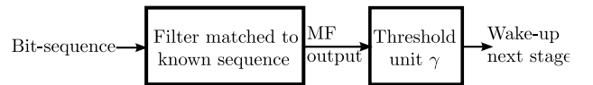
Fig. 5. Block diagram of a detector consisting of a matched filter (MF) and a threshold unit.
