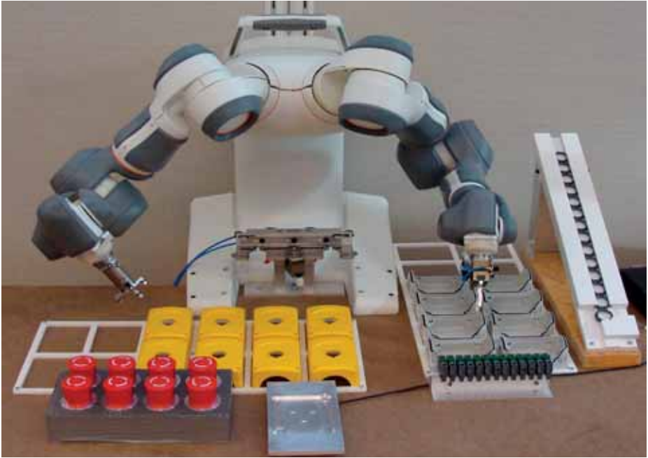
The FRIDA robot and the setup for the emergency stop button assembly.
