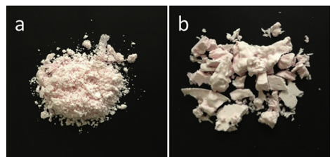
Fig. 8. Dried solid shea nut oil emulsion powders, a. non heated freeze-dried double emulsion left and b. heated freeze-dried double emulsion on the right.
