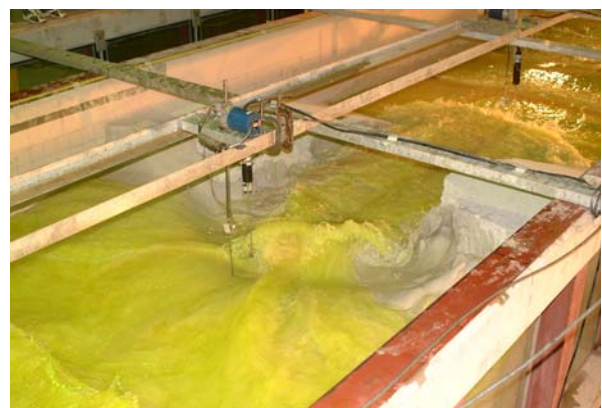
Figure 2-16. Supercritical flow into washover throat, hydraulic jump at bottom, widening of throat (Photos taken by Ken Connell)
