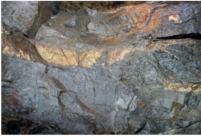
Fig 18 Chalcopyrite remobilisation Chalcopyrite filled fractures in the west wall of Malmkyrkan, Kleva gruva. Fracture width is c. 10 cm.
