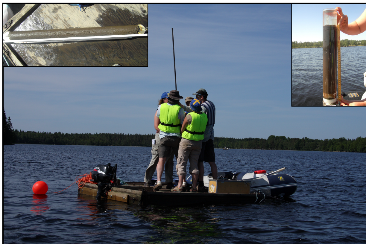
Figure 2. Sediment sampling in Lake Fiolen and examples of retrieved Russian and gravity cores.
