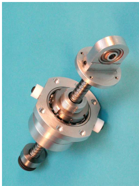
Mass \approx 1 kg, Inertance (adjustable) = 60–180 kg
