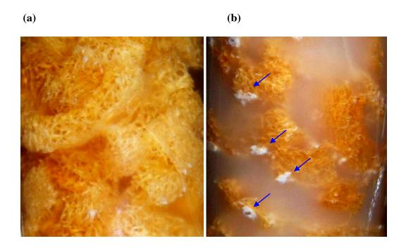
**Figure S3.** Packed-bed column with PEI-treated Poraver showing the immobilization matrix with immobilized cells of *P. acidipropionici* DSM 4900 during propionic acid production from glycerol.
