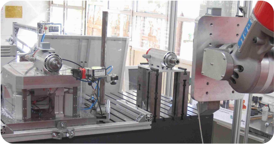
Figure 2.11 Experimental setup for evaluation of the effectiveness of the proposed micro manipulator, which is seen to the left. The machining spindle to the right is rigidly attached to the base. This setup is utilized for milling experiments without compensation.
