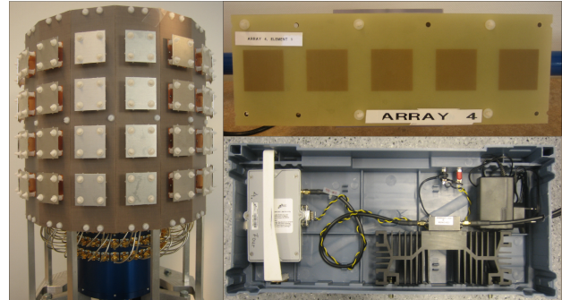
Fig. 1. (Left) MS antenna with 64 dual-polarized patch antenna elements. (Top right) BS ULA antenna with 5 dual-polarized patch antenna elements. (Bottom right) Transmitter module showing an OZ816 optical receiver unit and the ZVE-8G-7+ RF power amplifier.
