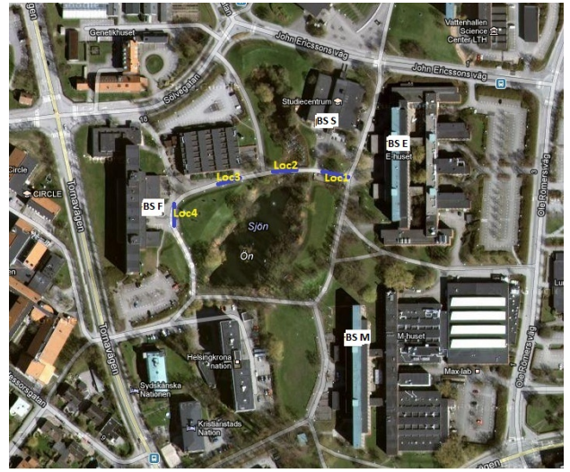
Fig. 3. Google Map photo of the measurement campaign area. Base station locations are indicated by labels BS E, BS S, BS F and BS M. The intended measurement route is plotted in blue color.
